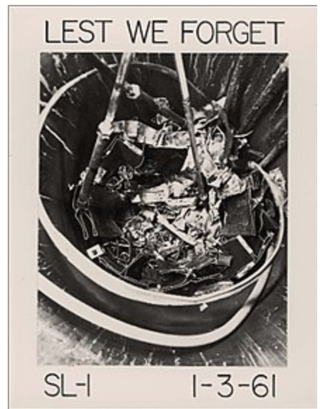
This image of the core from the SL-1 disaster, Idaho Falls, Idaho, USA , served as a reminder of the necessity for proper reactor practice and safeguards.
