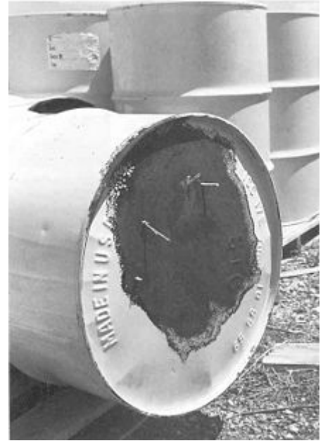
Corroded and leaking 55-gallon drum, for storing radioactive waste at the Rocky Flats Plant , tipped on its side so the bottom is showing.
